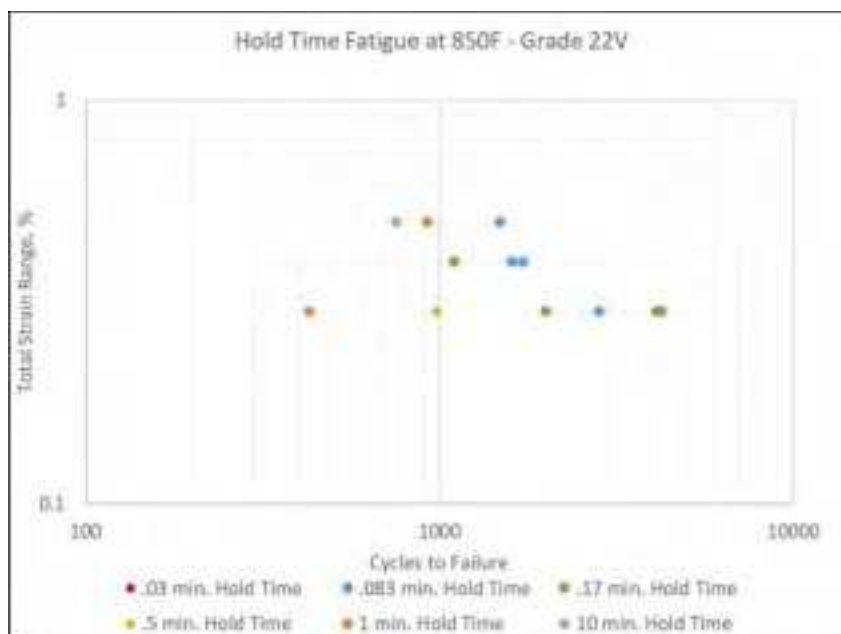
Figure 11-22: Grade 22V Hold Time Data (Creep Fatigue) for Grade 22V, Temperature of 850°F
