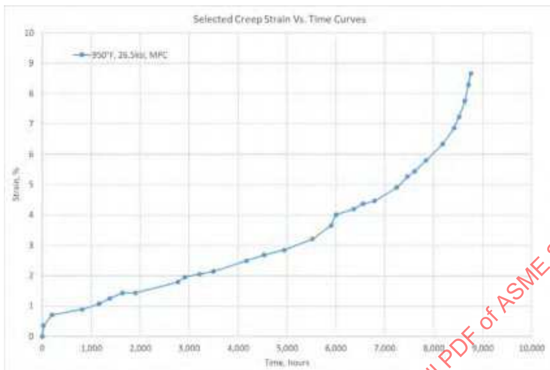
Figure 24-15: Short-Term Strain Vs. Time Data, (3Cr)
