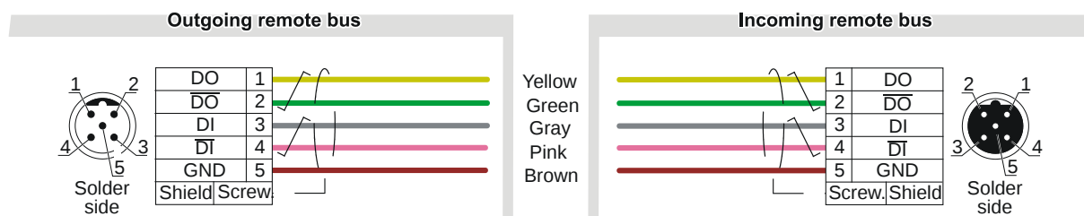
Figure A.5 – M12 circular connector pin assignments
