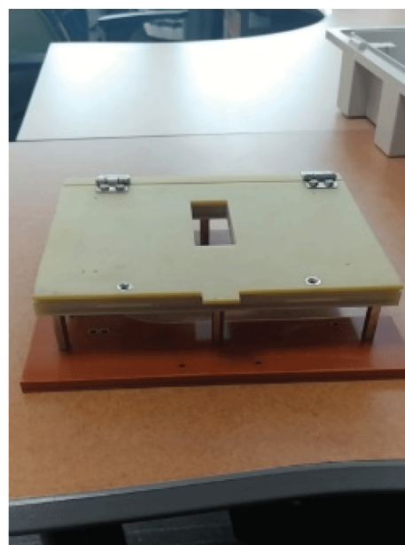
Figure 4 – Opened and closed sample jig
