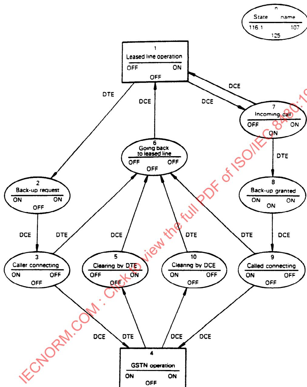
Figure 1 — Back-up Switching in "Direct Mode"
