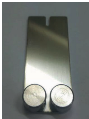
Figure A.3 — Bending tool for manual test
