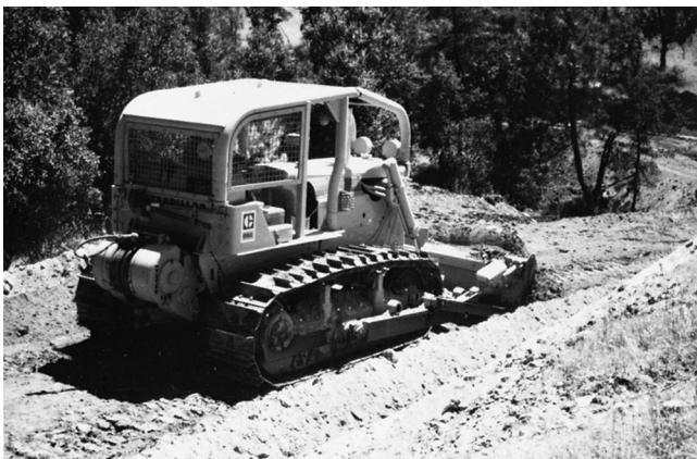
FIGURE A.5.1.3.2(3)(a) A Dozer Properly Equipped with Protective Canopy, Lights, Brush Guards, and a Winch.
