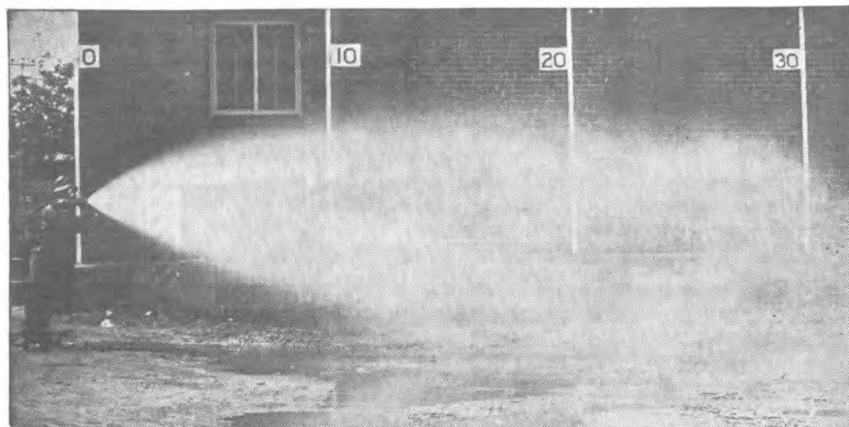
11.30. A spray nozzle discharge showing the pattern of the spray. Numbers on wall indicate distance from nozzle in feet.
