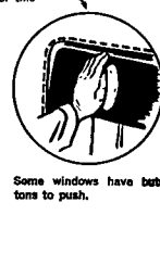
Figure A-1. The principal points to consider in gaining access to civil transport aircraft. Each aircraft must be examined individually to know how doors and windows may be most easily opened from outside.
