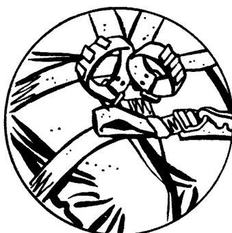
Figure B-15. Harness releases include lower leg restraints at the ankles (pull release pins at rear of ankle straps), upper leg restraints at left knee, lap belt, shoulder and crotch harness straps. Disconnect also oxygen hose and mike cord.
