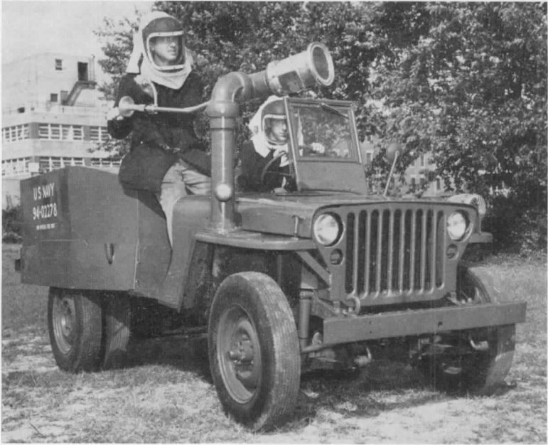
Fig. 4. Experimental Navy "Jeep" foam rescue vehicle carries 230 gals. of water and 20 gals. of foam. Designed for carrier operations.
