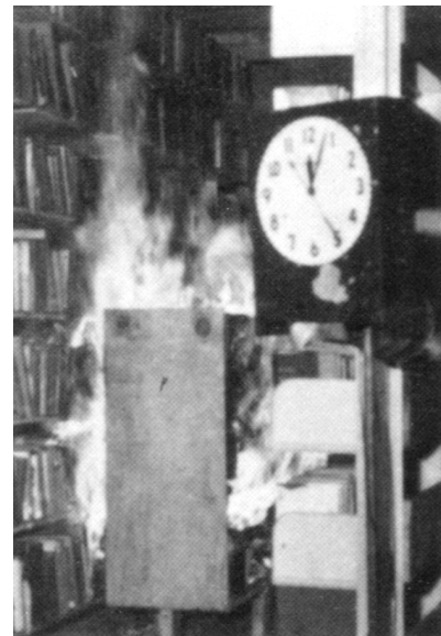
Figure J-2(c) Three minutes, 25 seconds; active burning in first tier; sprinklers not yet operating.
