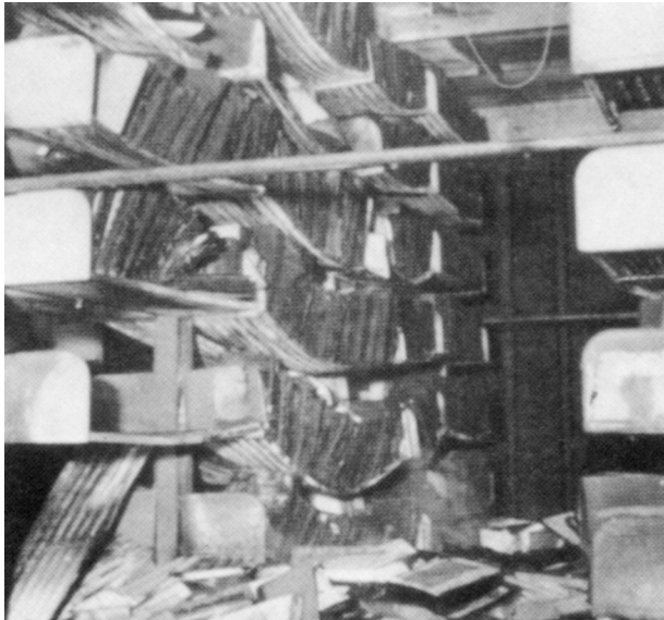
Figure J-3(g) Extent of damage to shelving after Test 2 (no sprinklers) on second tier, right aisle. Note severe charring of books and collapse of shelving.
