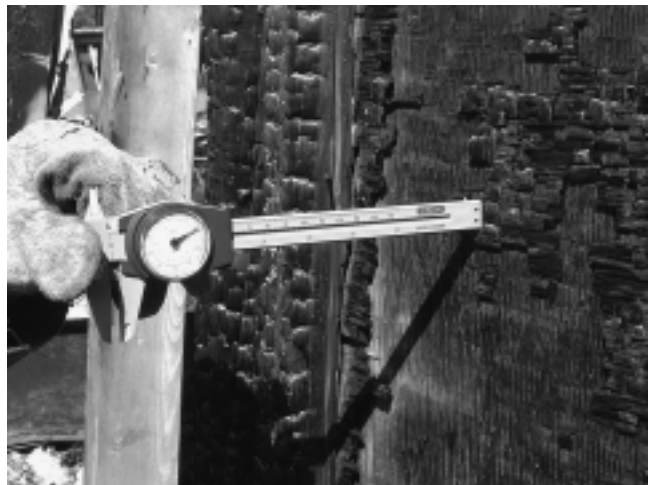
FIGURE 4.5.3.3(c) Using dial calipers to measure depth of char.
