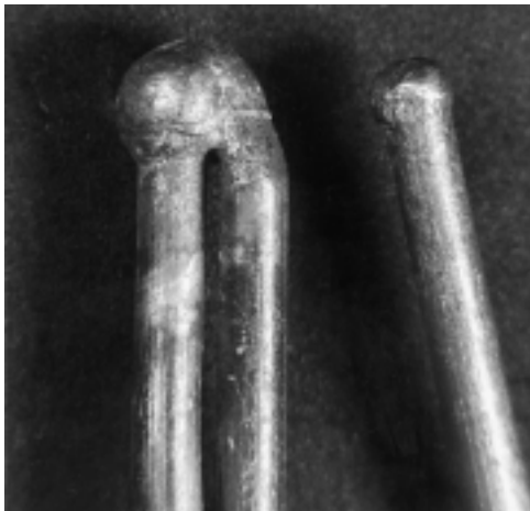
FIGURE 6.10.3(b) Copper conductors severed by arcing through the charred insulation with a large bead welding the two conductors together.
