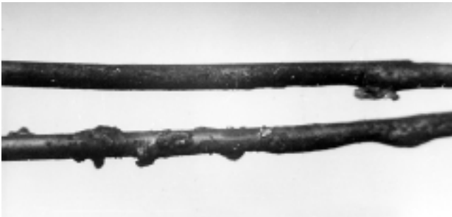
FIGURE 6.10.6.2(b) Fire-heated copper conductors, showing globules.
