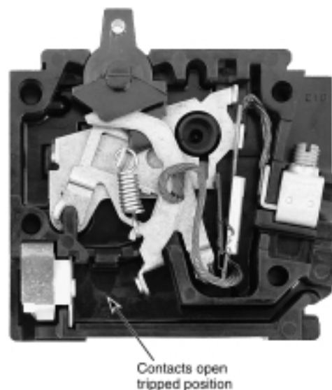
FIGURE 6.6.2(c) A 15 A residential-type circuit breaker in the open (tripped) position.
