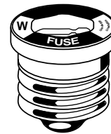
FIGURE 6.6.1(a) A typical, Edison-based nonrenewable fuse, single element, for replacement purposes only.
