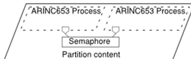
Figure 9 - Graphic representation of an ARINC 653 semaphore usage across two ARINC 653 processes
