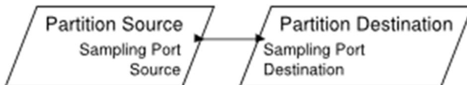
Figure 5 - Graphic representation of an ARINC 653 sampling port connected through two partitions
