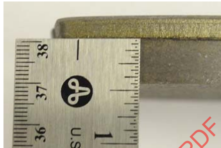
FIGURE 1 - MEASUREMENT OF FRICTION MATERIAL THICKNESS
