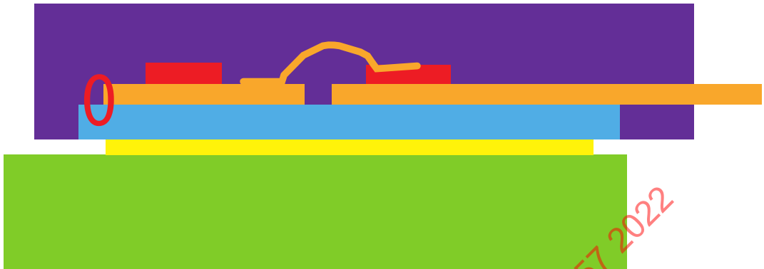
Figure B.4 Molded device with ceramic insulation
